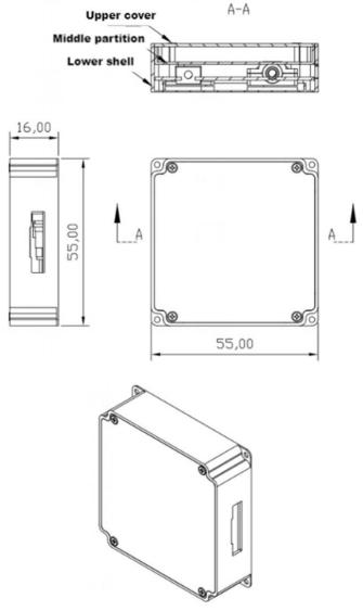
Note: The above is the standard size of 55\*55\*15mm. Customized structures such as special-shaped and open structures that are easy to integrate can be provided according to customer needs.
