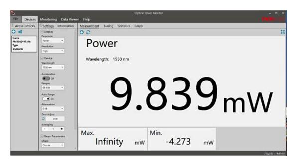
Laser power before connecting to fiber patch cord
