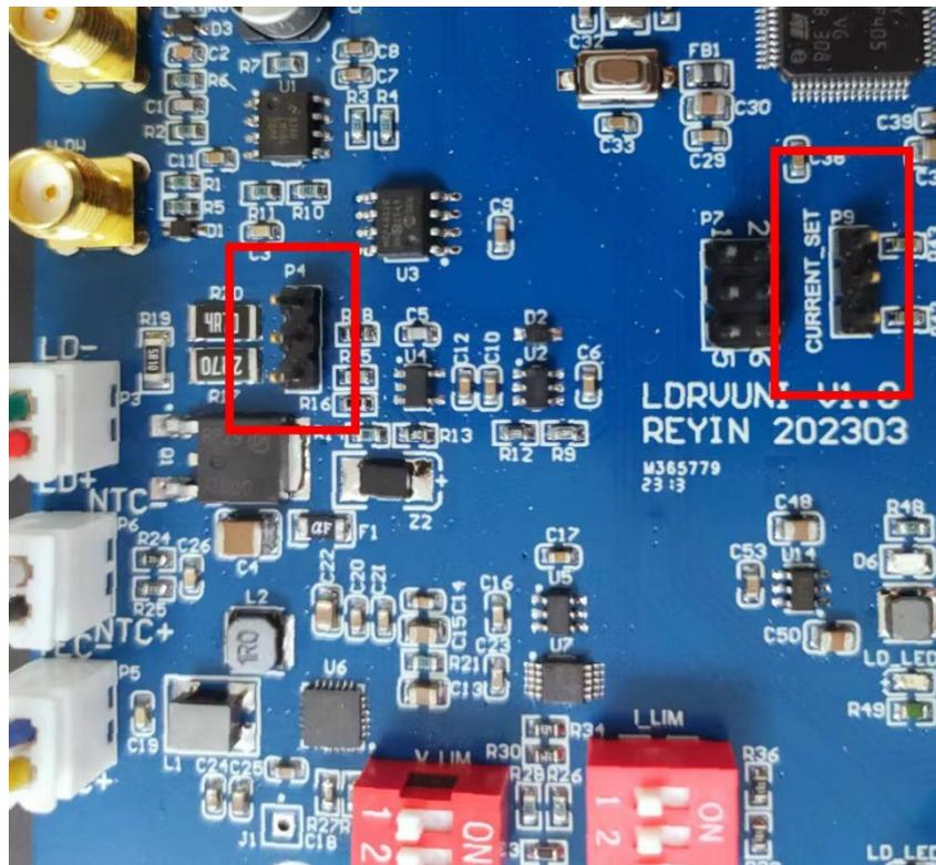
On the circuit board, P4 and P9 (CURRENT\_SET) are used to set the maximum current range of the circuit board. Note that the jumper positions on both must be exactly the same to ensure correct settings.
