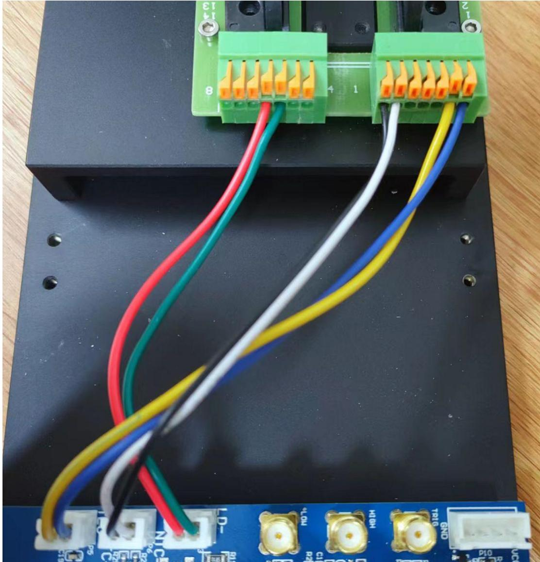
Connect the laser leads according to the markings on the circuit board and different laser mounting seats. After installing the laser, carefully check the connections again before powering on.
