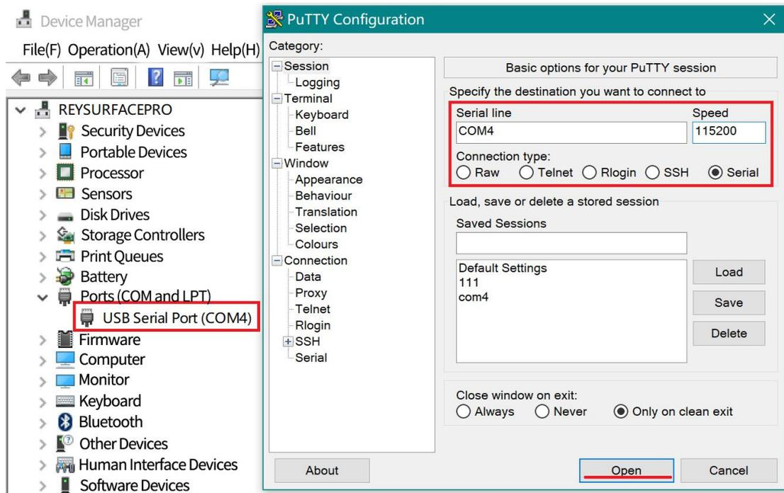
The computer acts as the master control (host), sending string commands. Each command begins with a colon (":") as the starting symbol, and ends with a carriage return (\r\n). After the lower machine executes the command, it will return a response. All functions can be accessed through the accompanying software. It is recommended to use the LDPD software to complete the settings and obtain the correct waveform, then click Save to store the parameters in the lower machine,
