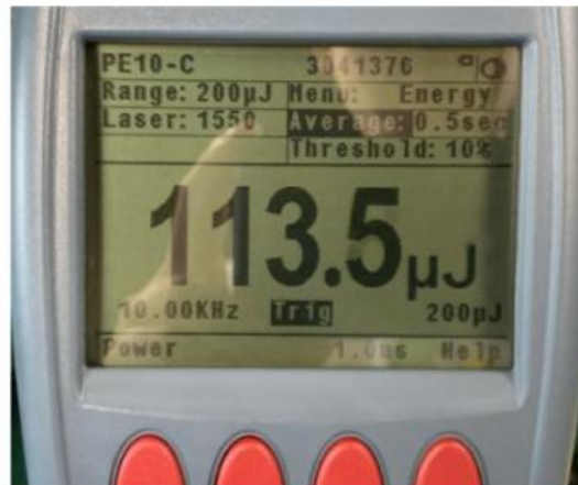
Pulse width test and pulse energy test @ 10kHz, 3ns.
