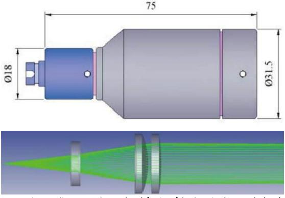
Beam waist spot diameter: Taken at the  $1/e^2$  point of the Gaussian beam, calculated using the theoretical value for single-mode fiber at each wavelength.
