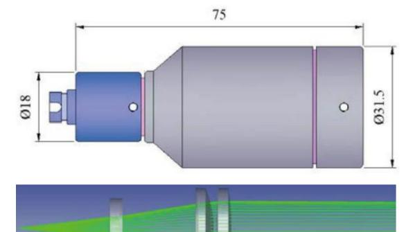
Beam waist spot diameter: Taken at the 1/e² point of the Gaussian beam, calculated using the theoretical value for single-mode fiber at each wavelength.
