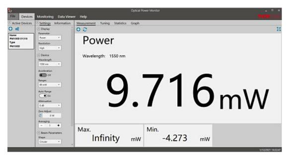
Power after connecting the fiber optic patch cord
