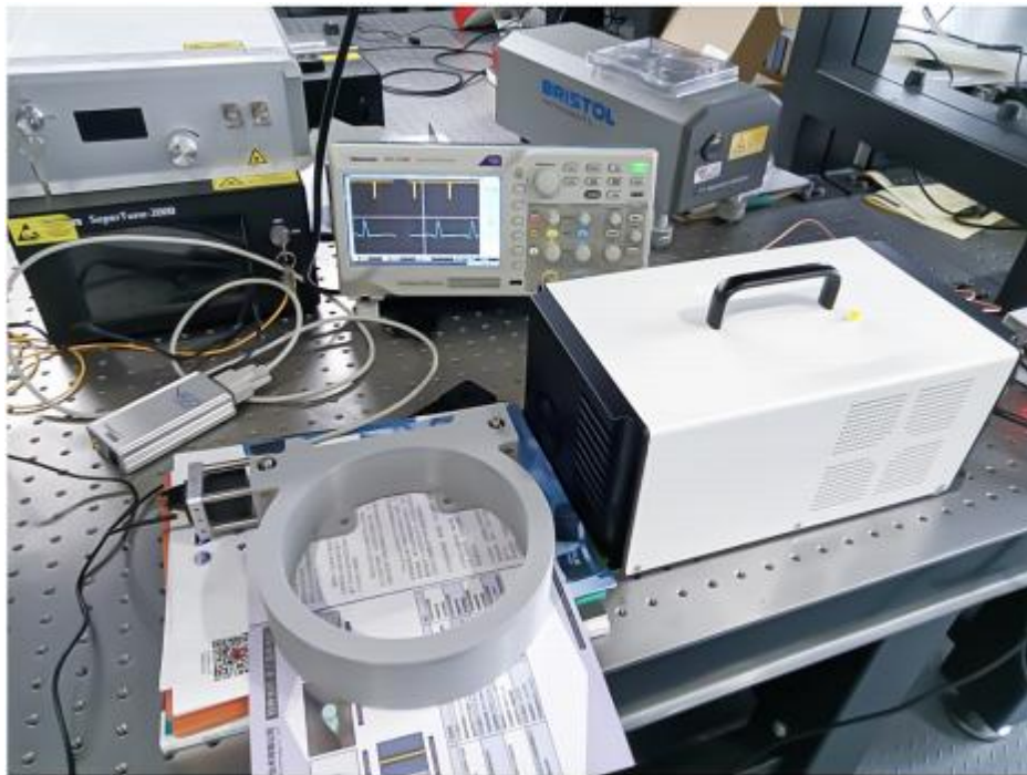
NF3 gas absorption measurement experiment system diagram
