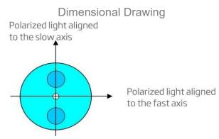
The default alignment mode of Idealphotonics' optical polarization-maintaining components is slow-axis alignment.
